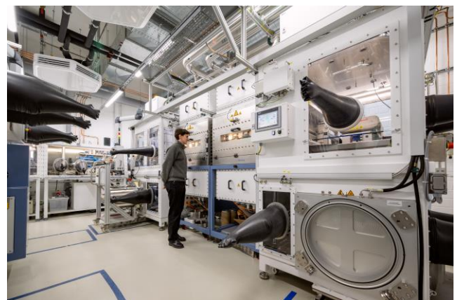
Figure 3: Experimental coating and drying system for electrodes in an argon atmosphere (Image source: TUM / Andreas Heddergott)
